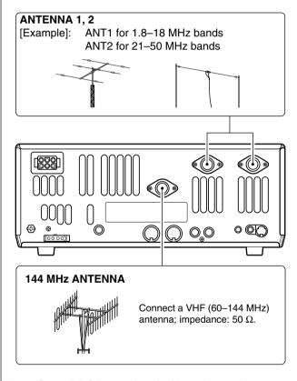
Your IC-746PRO is equipped with an internal antenna tuner (ATU) for operation on 160–6 m. This ATU is designed to work with an unbalanced 50  $\Omega$  feedline. The purpose of the internal antenna tuner is to match the impedance of your antenna system to as close to a 50  $\Omega$  load as possible. This ATU will not operate with a long wire or ladder line (450  $\Omega$  or other balanced feedlines). An external ATU such as the AH-4 would be necessary for this kind of operation.
