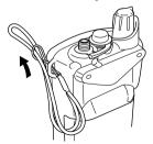
Pass the handstrap through the loop on the top corner of the transceiver as illustrated at left.
