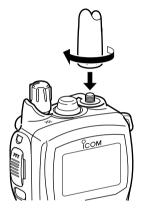
Connect the supplied flexible antenna to the antenna connector.
