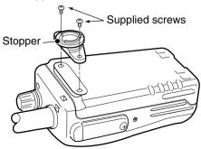
② Clip the belt clip to a part of your belt and insert the stopper to the belt clip.
