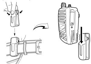
③ Once the transceiver is locked in place, it will swivel 360 degrees.
