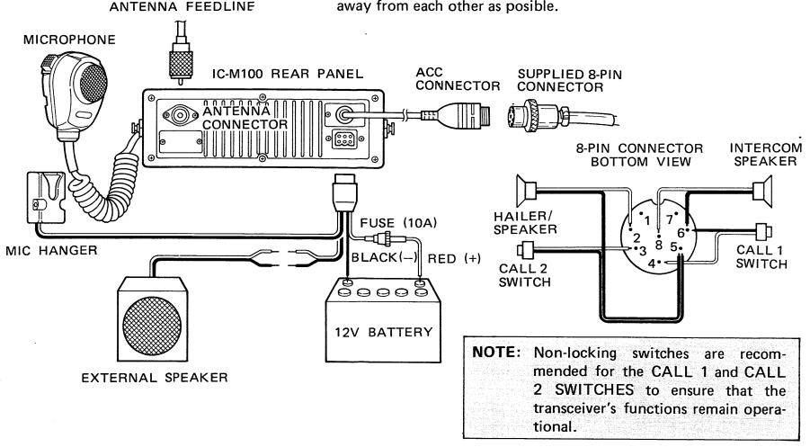
2 - 2 MOUNTING THE TRANSCEIVER The universal bracket supplied with your transceiver allows "over" or "under" mounting. Install the bracket so the unit is adequately supported, thus protecting it from wave shock and excessive vibration.
