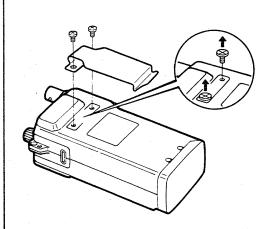
The belt clip allows you to attach the transceiver to your belt.
