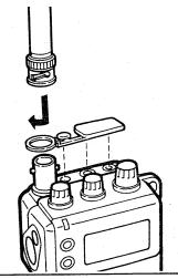
Attach the rainproof cap before connecting the antenna when desired.
