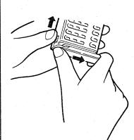
Push the bottom cap release button upwards, then slide the bottom cap to the right with the transceiver facing you.
