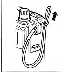
The handstrap allows you to easily carry the transceiver. Attach the handstrap as shown in the diagram at left.
