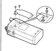
The belt clip allows you to attach the transceiver to your belt.
