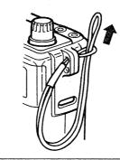
The handstrap allows you to easily carry the transceiver. Attach the handstrap as shown in the diagram at left.
