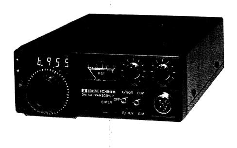
Congratulations on your purchase of the ICOM IC-245. The IC-245 is unique in its mobility, flexibility and compact size. Outstanding performance capabilities are produced by the proprietary ICOM C MOS LSI built into each IC-245. By itself, the IC-245 gives full command of the 144—148MHz 2 meter band. Add the sideband adapter and the IC-245 is a multimode 4MHz FM, USB, CW unit. Carefully reading this manual will help you get the most pleasure and effective use from your new transceiver.
