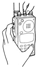
**CAUTION:** Resetting the CPU will clear and initialize all memory channel contents, SET mode settings, DTMF memory contents and clock and timer settings.
