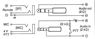
The above diagram does not apply when a condenser microphone is connected.
