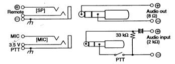
The above connection does not apply when a condensor microphone is connected.
