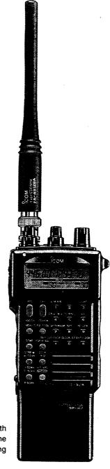
The photo shows IC-X2A with BP-82 BATTERY PACK. The battery pack differs according to versions.
