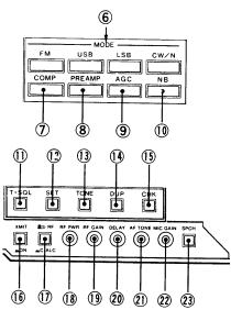
② AF GAIN CONTROL ③ SQUELCH CONTROL PHONES JACK **5 MIC CONNECTOR 6 MODE SELECT SWITCHES** TSPEECH COMPRESSOR SWITCH ® PREAMP SWITCH **MNOISE BLANKER SWITCH ®TONE SQUELCH SWITCH ® TONE SET SWITCH** (3) SUBAUDIBLE TONE FREQUENCY/ TONE CALL (IC-275E) SWITCH ① DUPLEX SWITCH ③ DUPLEX CHECK SWITCH () TRANSMIT/RECEIVE SWITCH **METER SWITCH** ®RF POWER CONTROL @RF GAIN CONTROL
